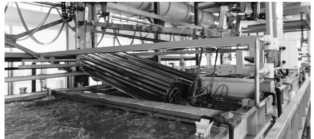
Automated aluminium anodizing
